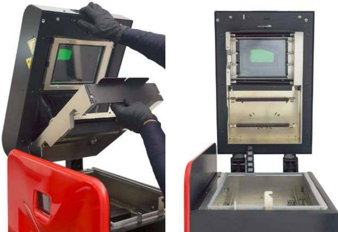
Image. Correct placement of the laser protection glass on the heater module.
