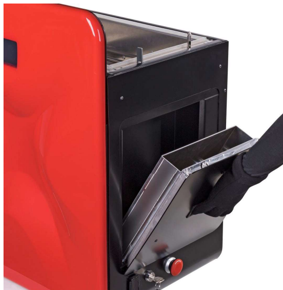
Image. Removing the remaining powder from the inside of the printer.
