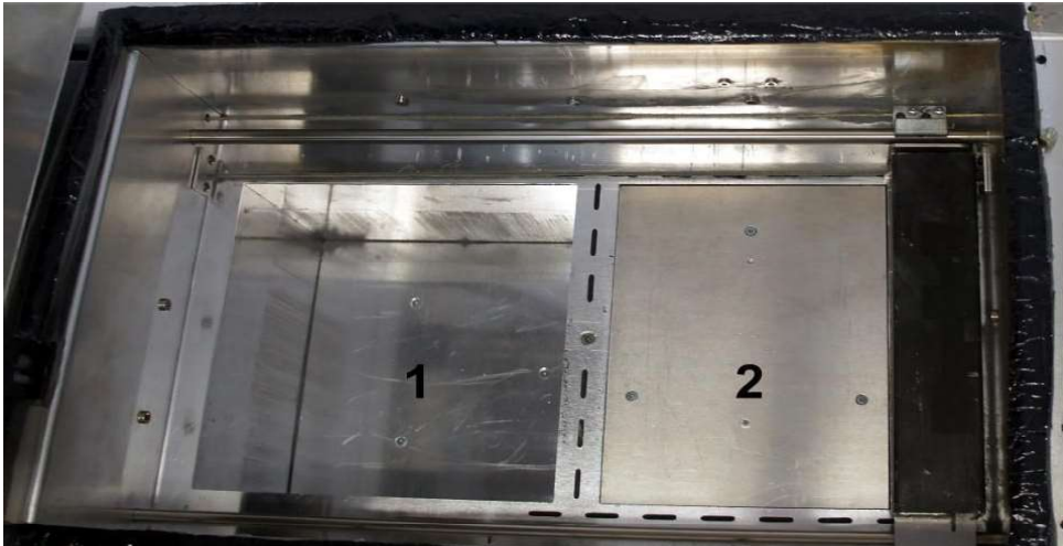
Image. Positioned Beds, ready to be filled with powder and the base position for the Recoater.
