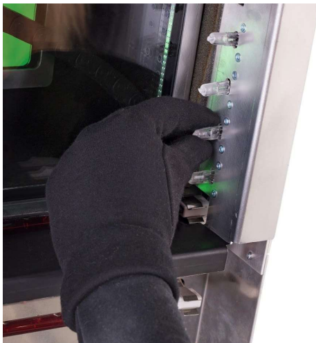
Image. Correct removal of the old and installing the new infrared heaters.
