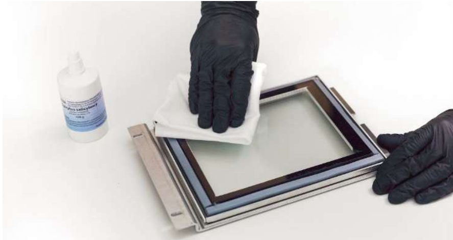
Image. Cleaning the laser protection glass
