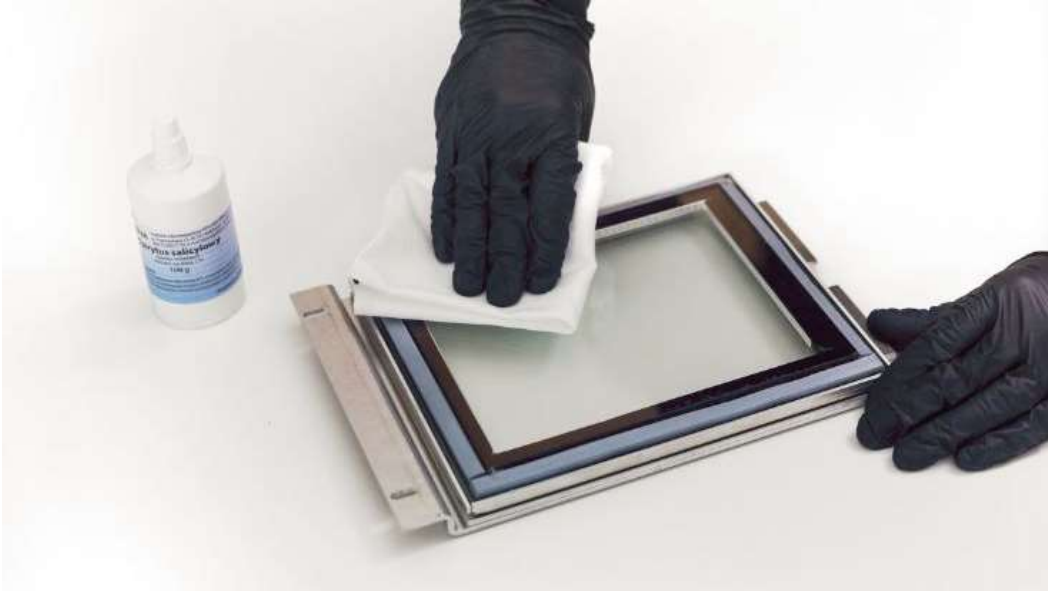
Image. Cleaning of laser protection glass
