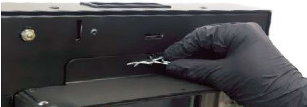
Image. heater module - split pin system
