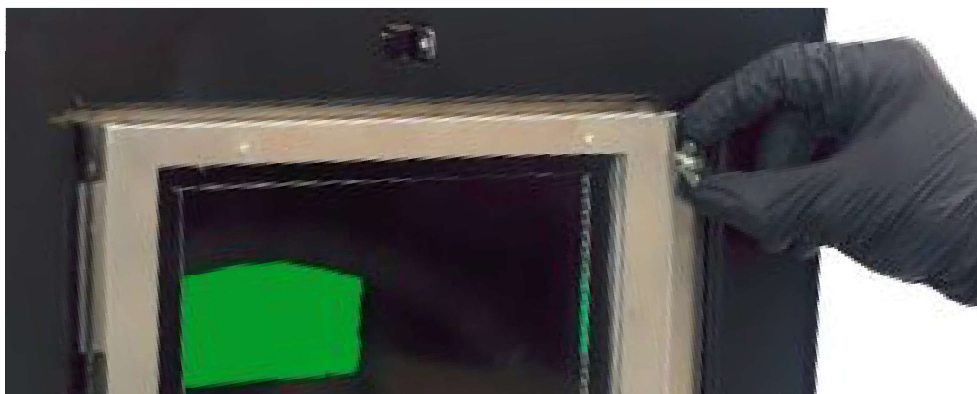
Image. Correct placement of the laser protection glass on the heater module.
